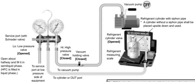
The R22 liquid refrigerant contained in the 1/4 charging hose from the manifold to the equipment service port shall be calculated as about 20 g/m (at  $20^{\circ}$ C).
