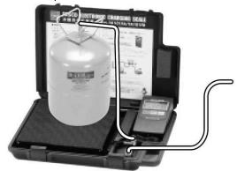
When the minus value shown in the indicator has reached the specified quantity to be filled, close each valve and remove the charging hose.
