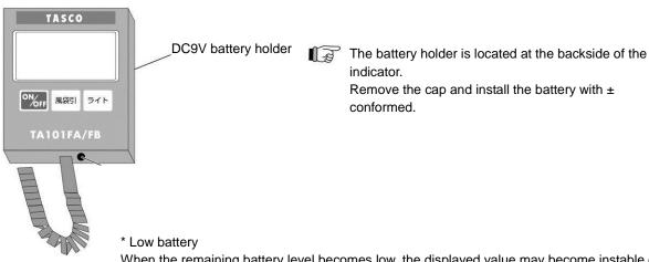
When the remaining battery level becomes low, the displayed value may become instable or a wrong value may be displayed. As soon as the indicator displays mark, replace the battery with a new one.
